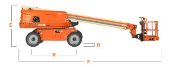
Platform Width 36-in / 0.91-m A. В. Platform Length 96-in / 2.44-m Machine Width C. 8-ft 2-in / 2.48-m D. Tailswing 4-ft / 1.22-m E. Machine Height 8-ft 2.4-in / 2.50-m F. Machine Length 28-ft 7-in / 8.71-m G. Wheelbase 8-ft 2.7-in / 2.5-m **Ground Clearance** H. 11.3-in / 29-cm
